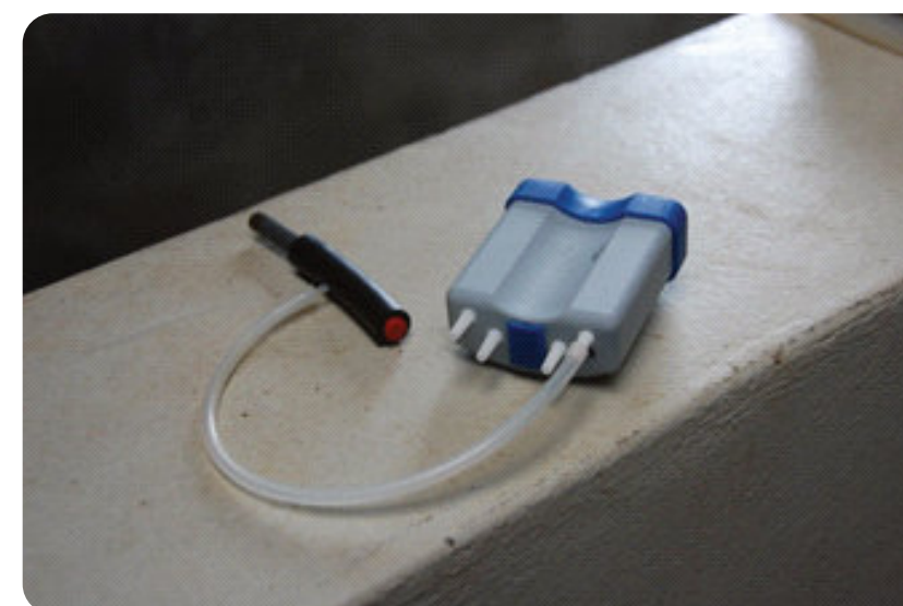
VaDia prepared for Falloff recording (measurement tube closed on one end)
