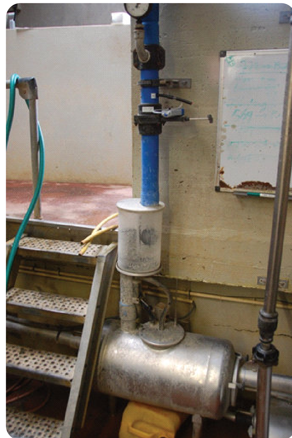
VaDia connected to the milk receiver at point Vm (exact test point may vary due to local legislation)
