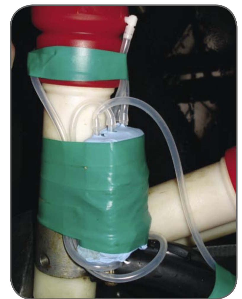
VaDia logger can be used on any type and brand of milking equipment, including robot
