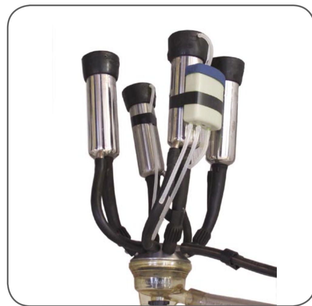
VaDia logs the vacuum at 4 points in the milking cluster
